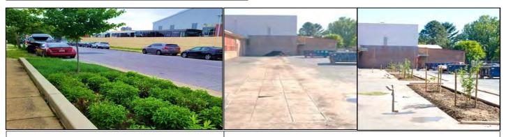
**Bioretention:** Micro-bioretention is a sunken area where plants and soil are installed to naturally filter polluted rainwater before releasing it slowly to storm drains and waterways, improving water quality.
